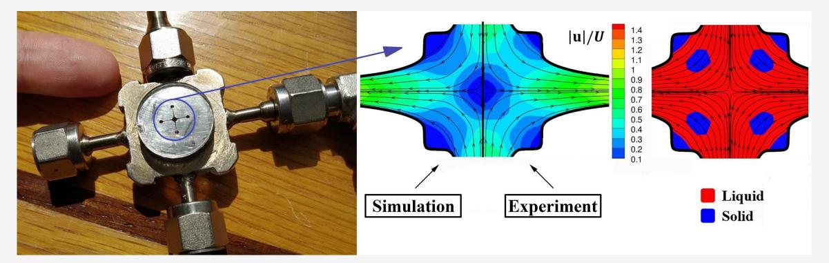
The results of the simulations matched the results of the experiments in OSCER microdevice. Credit: University of Patras
